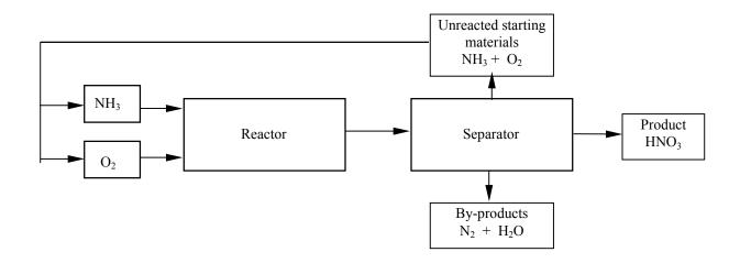
The reactant stream entering the reactor will be controlled so that it always contains 2 moles of  $O_2$  for every 1 mole of NH<sub>3</sub>, and the mixed reactants are to be pumped through the reactor at a rate of 1000 kg/h. Nitric acid is formed according to reaction #1 below. Unfortunately, an undesirable side reaction is also possible, as shown by reaction #2.
