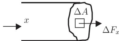
Figure 1.13: Force  $\Delta F_x$  Acting Over Small Area  $\Delta A$
